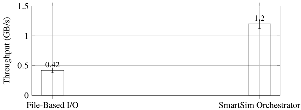
Figure 5: Data transfer throughput: SmartSim in-memory Orchestrator vs. file-based I/O (baseline). Means \pm standard deviation, 10 repetitions.
